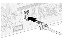
Connect the LAN cable with the device.
