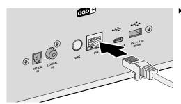
► Connect the LAN cable with the device.
