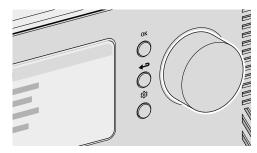
The device is controlled and operated using the navigation keys and the rotary control (e.g. to select menu items or follow the instructions on the display).
