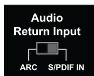
**S/PDIF In:** Audio from the device connected to the receivers **S/PDIF In** is sent to the matrix/transmitter over HDBaseT.
