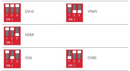
\* the 3.5mm audio input on the NHD-200-TX is only activate in DVI-D or VGA modes.
