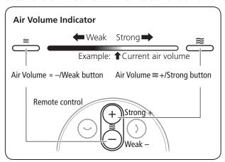
\* The Air Volume Indicator lamp changes right and left to indicate the current air volume.
