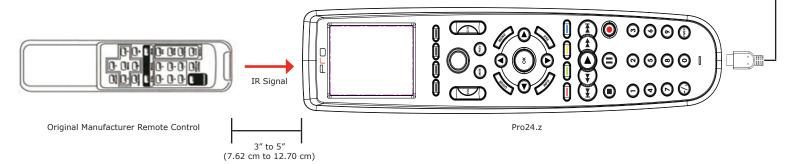
The Pro24.z is capable of capturing infrared codes from original equipment manufacturer remote controls. This IR learning capability is designed to work together with the Pro Control Studio library manager software. To capture infrared codes, follow the steps listed below:
