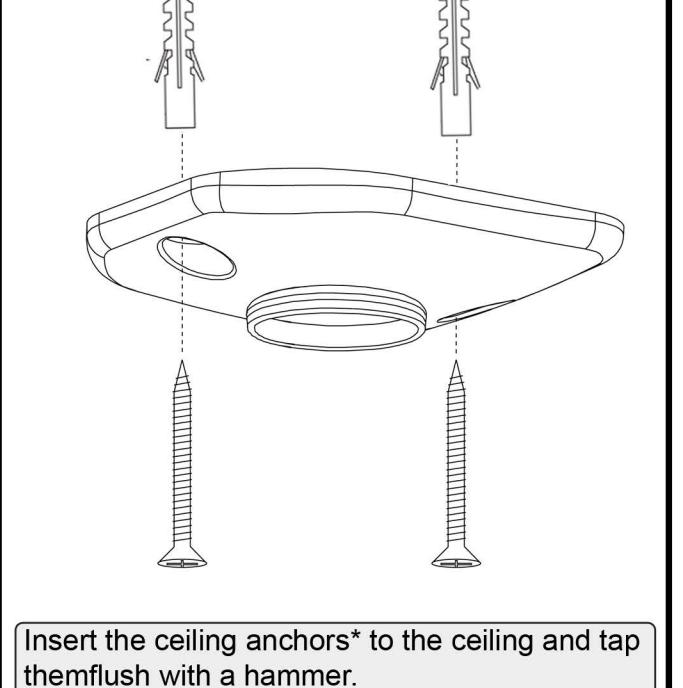
Insert the ceiling anchors\* to the ceiling and tap them flush with a hammer.
