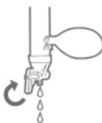
Step 3: Open the red water tap (vertical) and dispose the dirty water away from where it could come into contact with drinking vessels, cutlery, or other human contact.
