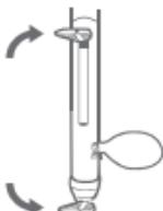
Step 1: Ensure there is water in the roll bag. Close BOTH the blue safe water tap and the red water tap (horizontal).
